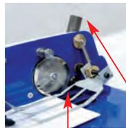
Strong self sharpening HSS steel blades. Variable adaption of the cutting width
